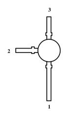
BF970 Marking Plastic case (~TO 50) 1= Collector; 2= Base; 3= Emitter
